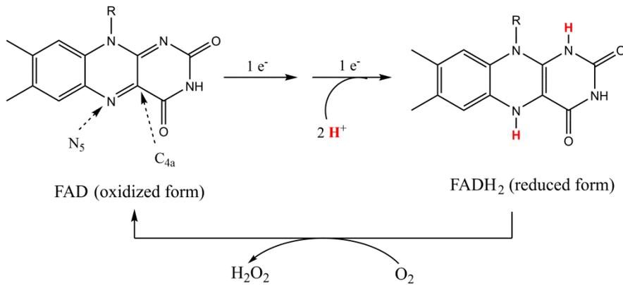
We did not discuss the detailed chemistry, but this reoxidation involves a  $C_{4a}OOH$  ( $C_{4a}$  hydroperoxide) intermediate and involves radical ( $1e^-$ ) chemistry.
